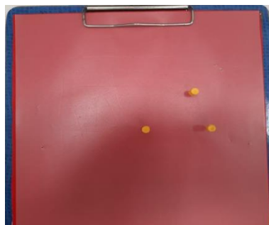
Figure 32: Three pins on the plastic sheet marking the three points of an angle
