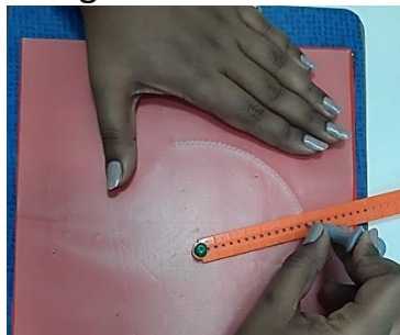
Figure 54: The WT ruler being used as a compass to draw a circle
