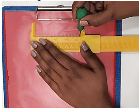
Figure 13: Connecting plotted points with the Squirrel ruler
