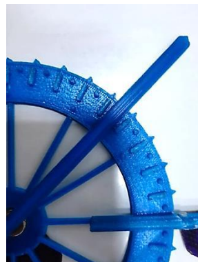
Figure 46: The Garg protractor with a line marker set at 45 degrees hiding the relevant tactile marking under it
